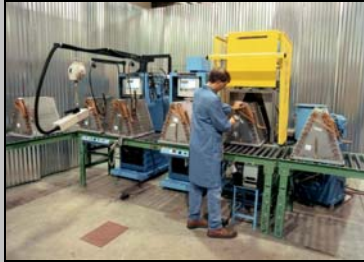
A-COIL STATION Integration of a "Gross test" and final Helium leak test minimizes production delays identifying large leaks early in the process
