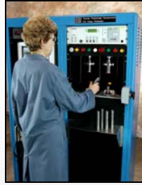
AIR-BAG INFLATOR TESTER Essential in providing critical test for safety component with confirmed disposal of parts that fail the test
