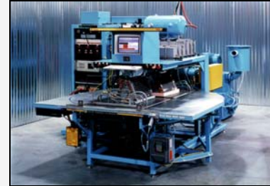
A/C COMPONENT TESTER System design with automated turntable system provides a cost effective solution to meet the throughput required by production
