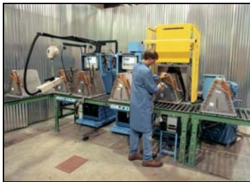
A-COIL STATION Integration of a "Gross test" and final Helium leak test minimizes production delays identifying large leaks early in the process
