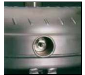
Calibrated leak built into torque converter
