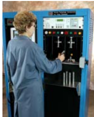
AIR-BAG INFLATOR TESTER Essential in providing critical test to 1x10^-5 atm-cc/s for key safety component with confirmed rejection.
