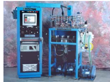
TERMINAL POST TESTER The lead-to-plastic interfaces of terminal posts for lead-acid batteries are helium leak tested.
