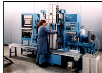
BATTERY CASE TESTER Inside-Out production tester for leak rate to 1x10^-4 atm-cc/s in production environment.
