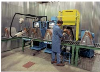
A-COIL TEST STATION A combination of Go-No-Go and final He leak test minimizes line delays identifying large leaks early.
