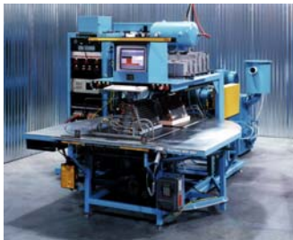
A/C COMPONENT TESTER Automated turntable system provides the throughput required by the production process.
