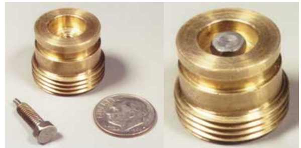
Stainless Steel Capillary Calibrated Leak built into a #10/32 bolt that is threaded into a drilled and tapped component of a Valve Module test part.
