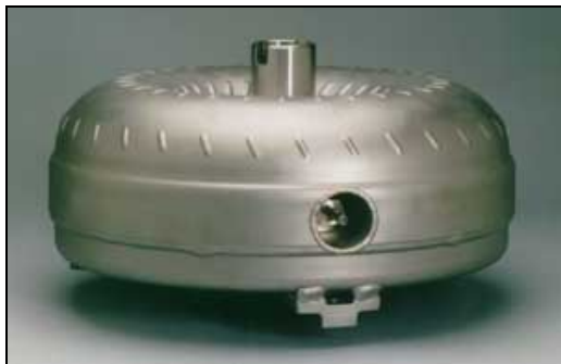
NIST-Traceable Calibrated Leak built into a well in a production test part for a Torque Converter. The threaded leak is removable / replaceable.
